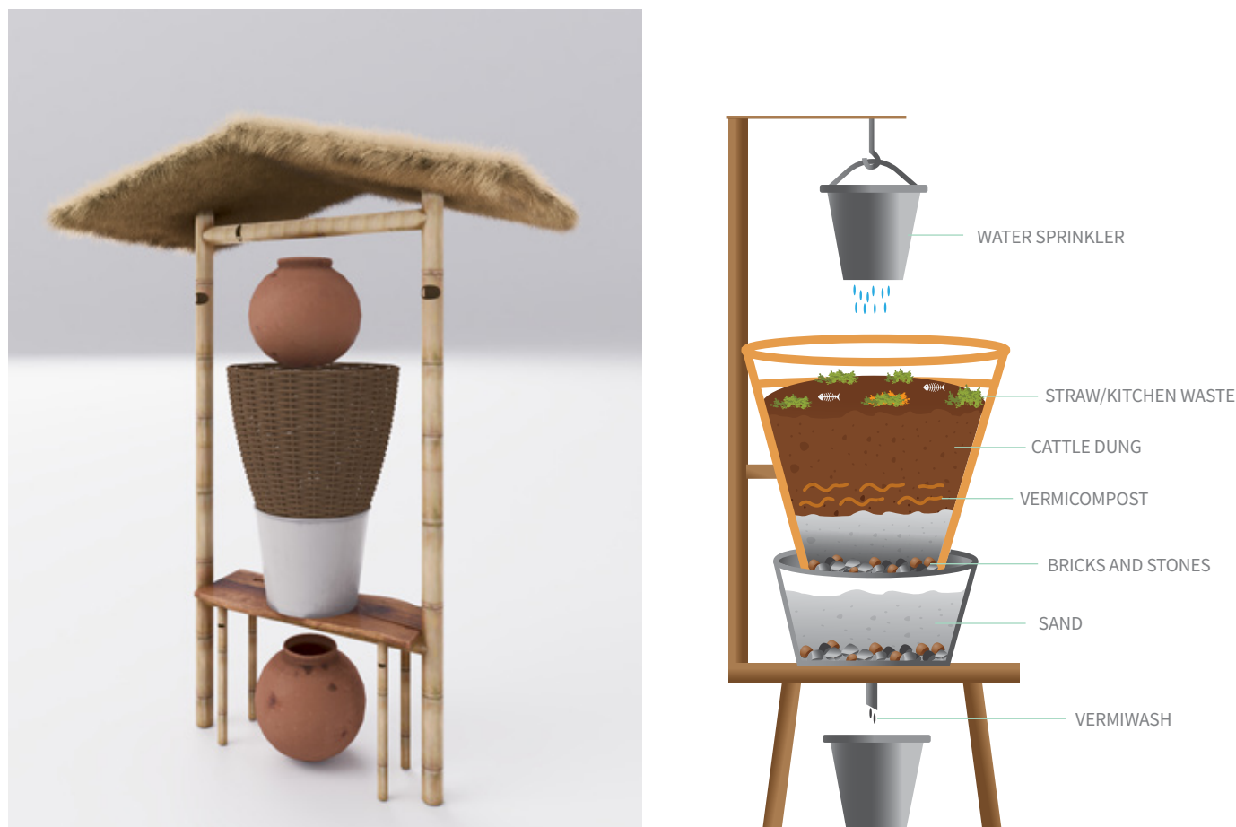
FIGURE 3 & 4: A MODEL OF A VERMIWASH SET UP AND A CROSS-SECTION SHOWING COMPONENTS AND MATERIAL.
