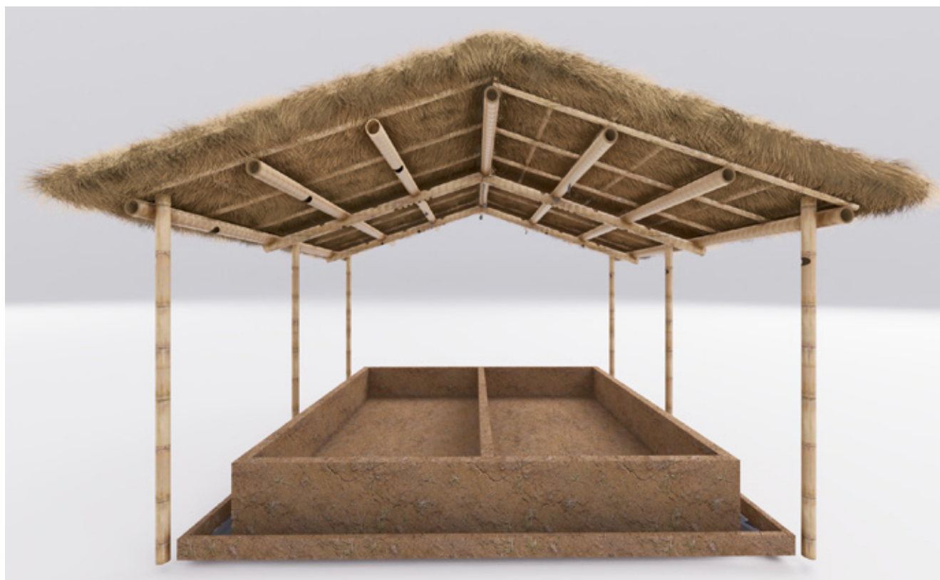
FIGURE 2: A MODEL OF A VERMICOMPOSTING SHED USING LOCAL MATERIALS
