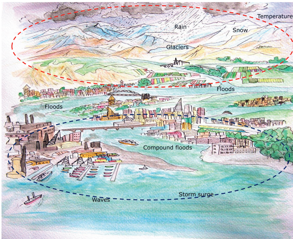
Figure 1.3: Schematic representation of different systems i.e. mountains (area within red dashed line where drivers of hazard such as extreme rain, high temperature, snow and glaciers melt components affect floods) and coastal environment (area within blue dashed line where drivers of hazard form mountainous catchment as well as storm surge and wave from sea affect floods) (sketch credit: Kriti Shrestha).
