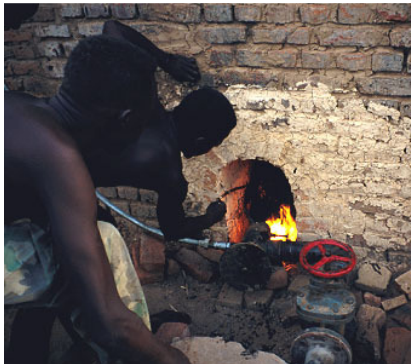
Figure 1: Brickmaker lighting a kiln with a liquid fuel burner.
