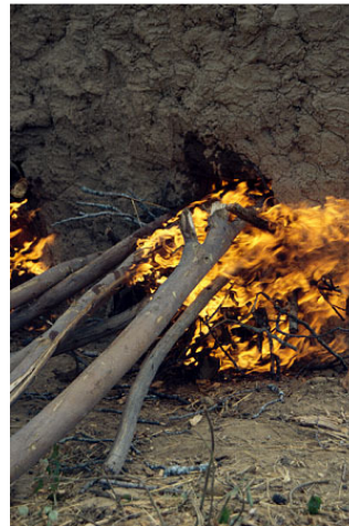
Figure 2: Firing bricks using wood as a fuel.
