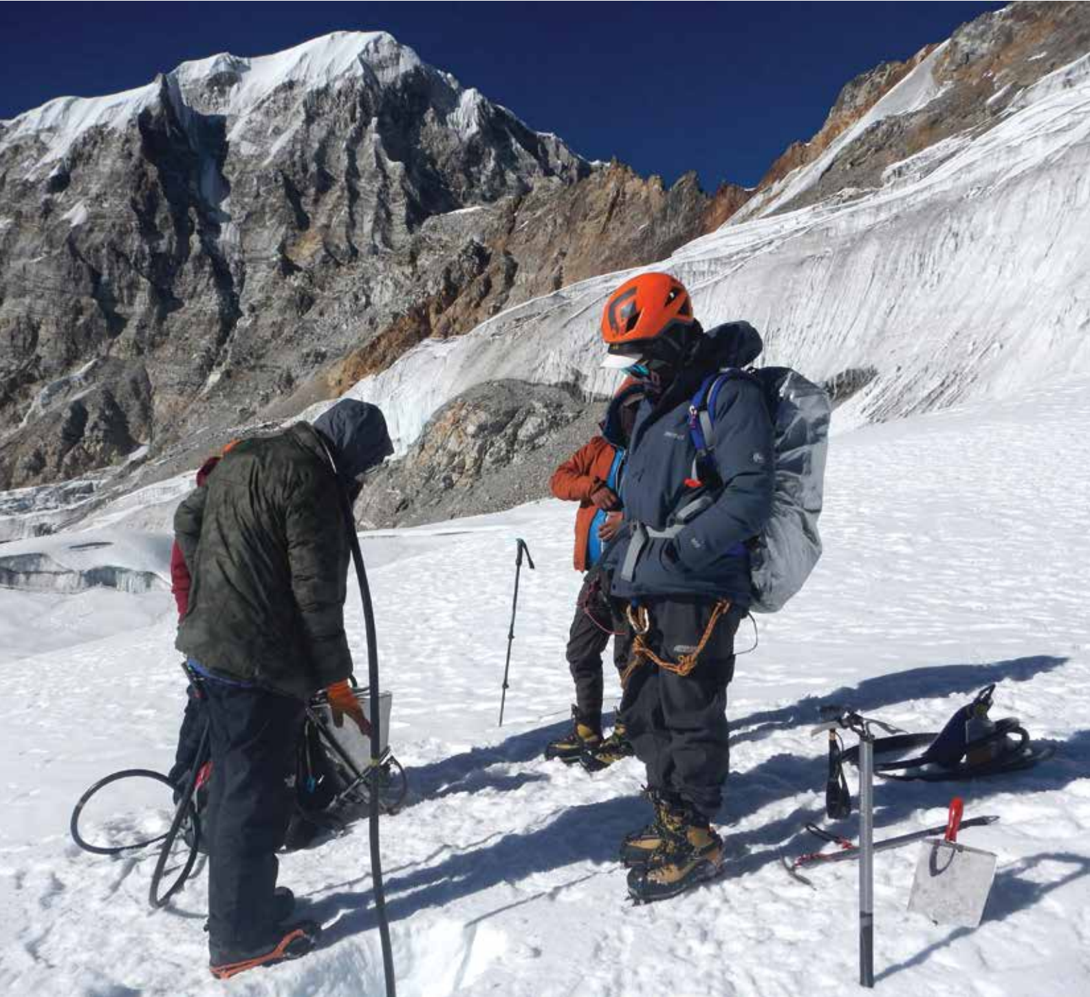
STREAM DRILLING ON THE YALA GLACIER FOR STAKE INSTALLATION
