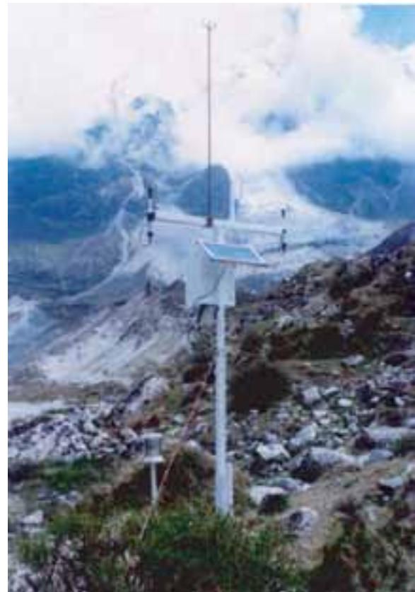
Figure 65: An automatic weather station equipped with a lake water-level recorder, Lirung, Nepal
