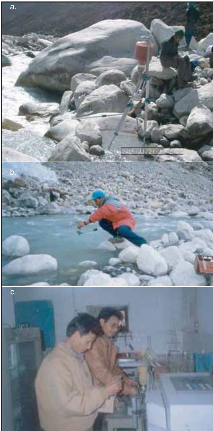
Figure 42: Discharge measurement using the dilution method: a. dye tracer injection using a Mariotte bottle; b. sample collection; and c. laboratory analysis of tracer concentration
