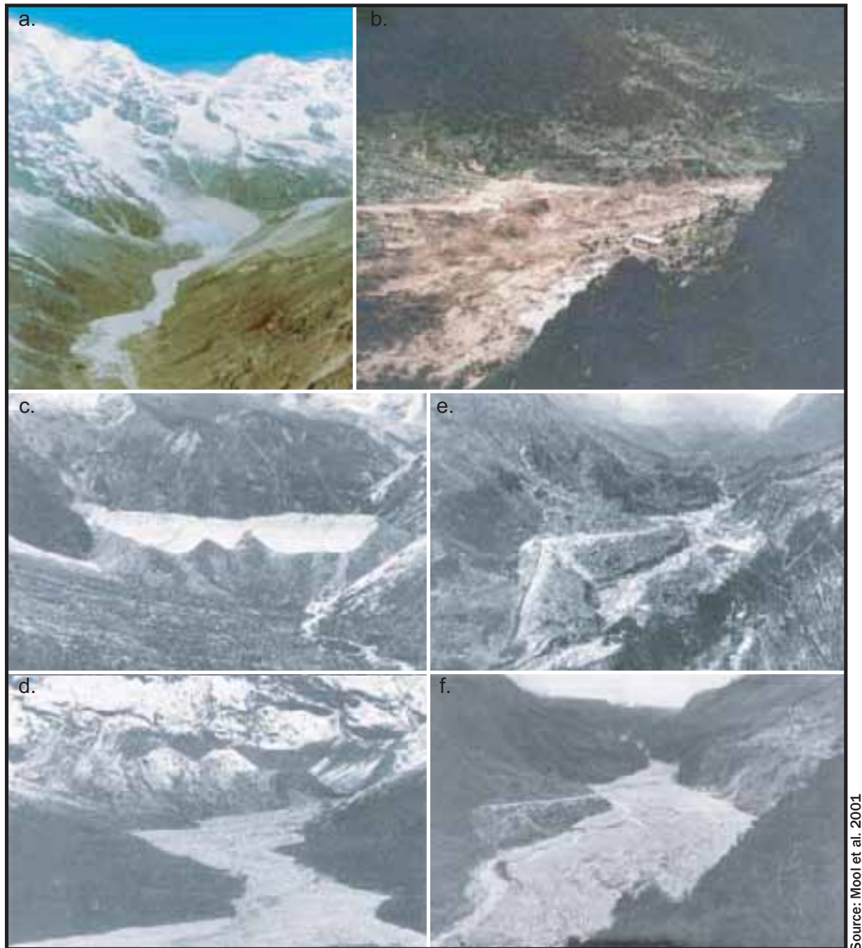
Figure 21: a. Dig Tsho lake after the GLOF outburst in 1985; b. the flash flood caused by the Dig Tsho outburst; c. the end moraine of Dig Tsho before the breach; and d. after the breach; e. the Namche hydropower station site before; and f. after the outburst
