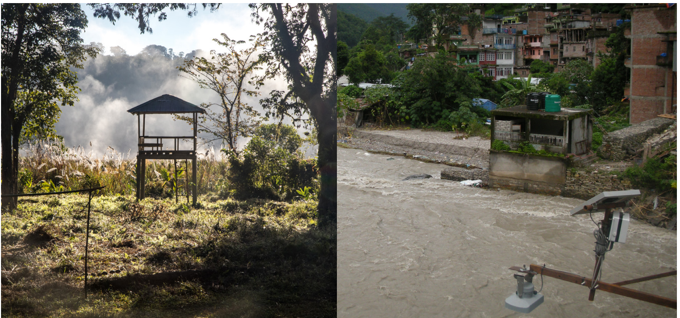
Left: Watchtower (also known as 'machan'); and Right: Radar sensor for water level observation
