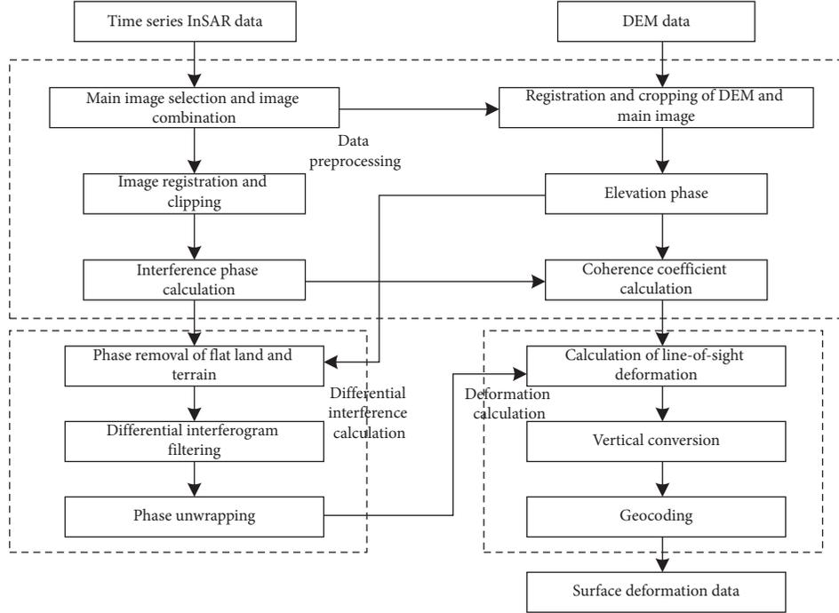
FIGURE 3: Flowchart of D-InSAR processing.
