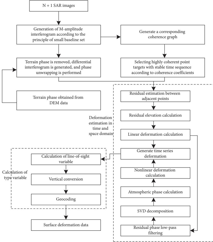
FIGURE 4: SBAS-InSAR data processing flow.
