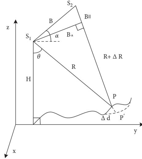
FIGURE 2: Geometric schematic diagram of two-orbit D-InSAR.
