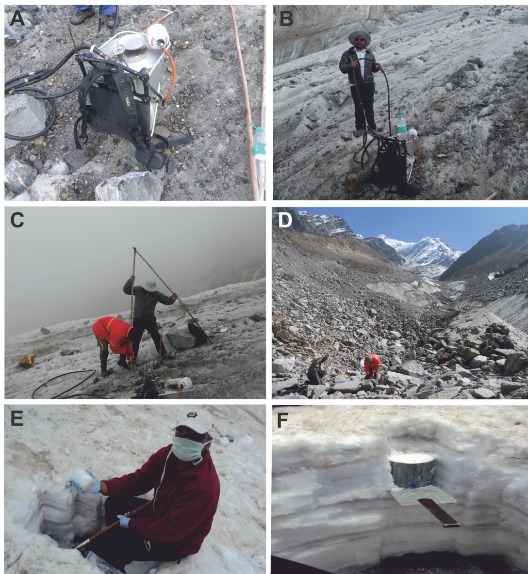
Fig. 2. Steam drill operation (panels (A) to (D)) for ablation stake networking on the Dokriani Glacier during October 2013. Panels (E) and (F) show snow pitting in the accumulation zone. The stakes were set up as per methodology proposed by several researchers (Østrem and Brugman, 1991; Dobhal et al., 2008, 2013; Cogley et al., 2011).
