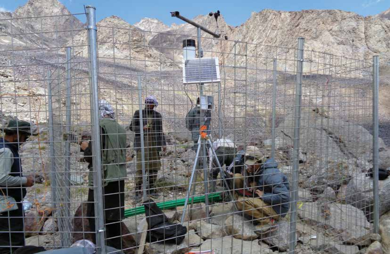
Installing an automatic weather station on Pir Yakh glacier, Panjshir valley.
