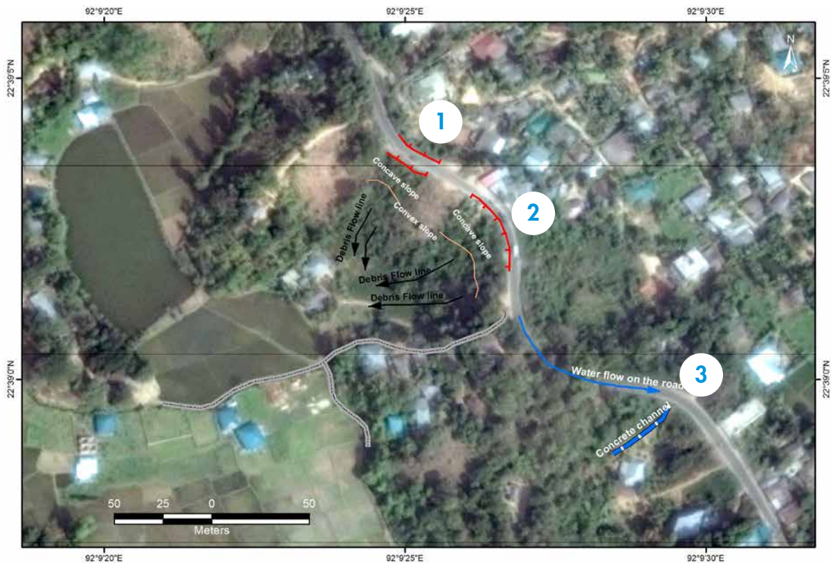
Figure 10: Plan view of saddle side slope failure at Monoghor-Rangapani at Ghagra bazar
