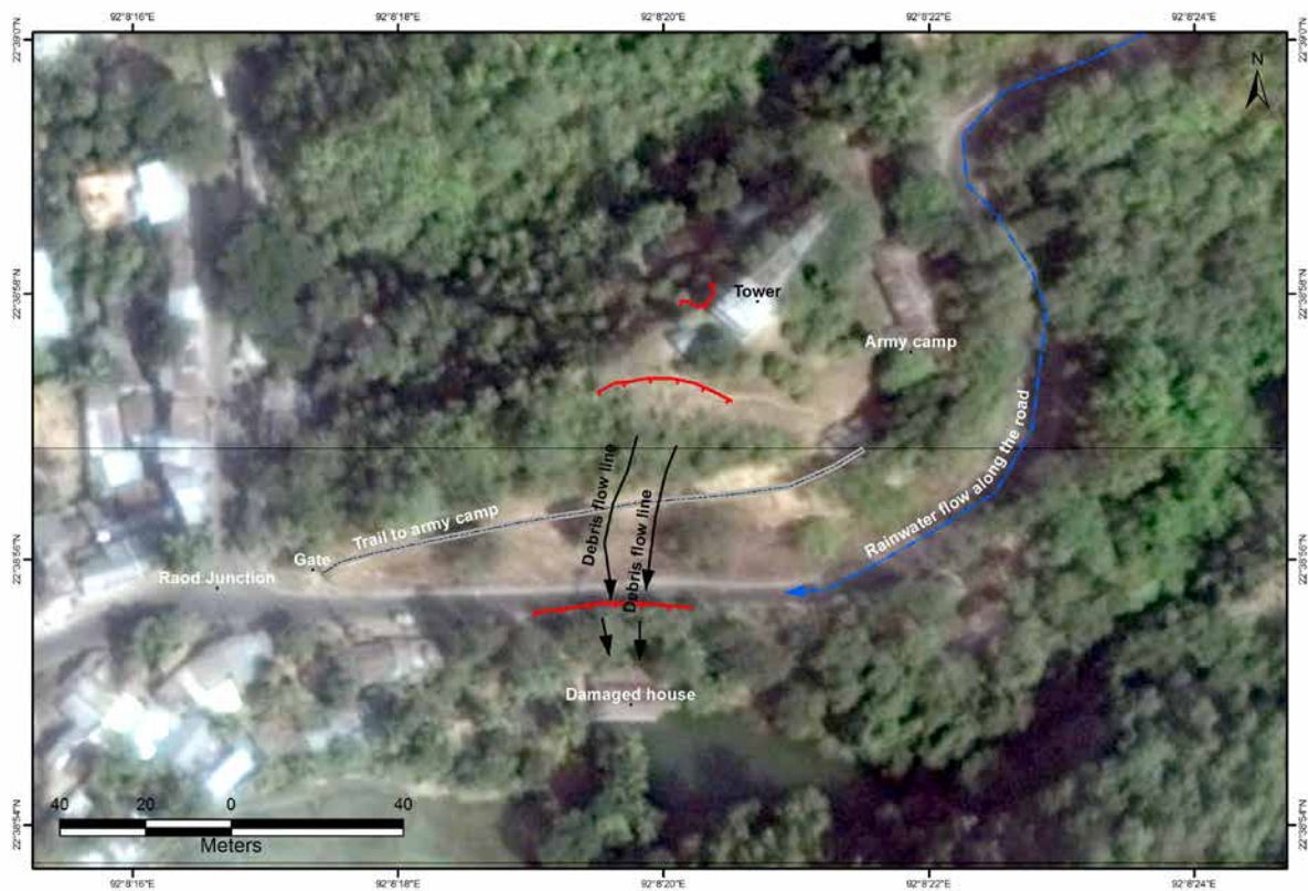
Figure 5: Plan view of hill slope failure at Manikchari Army Camp area
