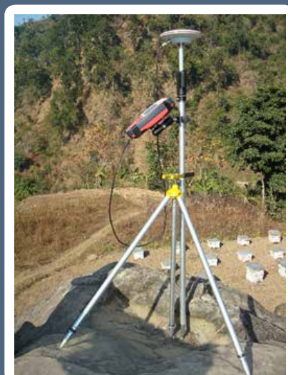
Figure 3: CFUG members delineating the community forest (left); differential global positioning system survey equipment (right)
