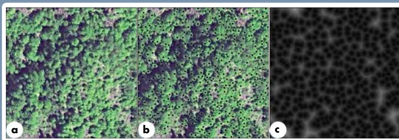
Figure 14: Delineation of crown projection area (CPA): a) satellite image, b) image with local maxima/tree tops, c) distance from tree tops
