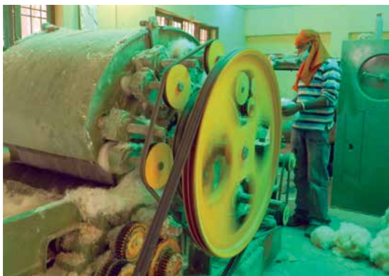
Carding of nettle fibre an improved machine
