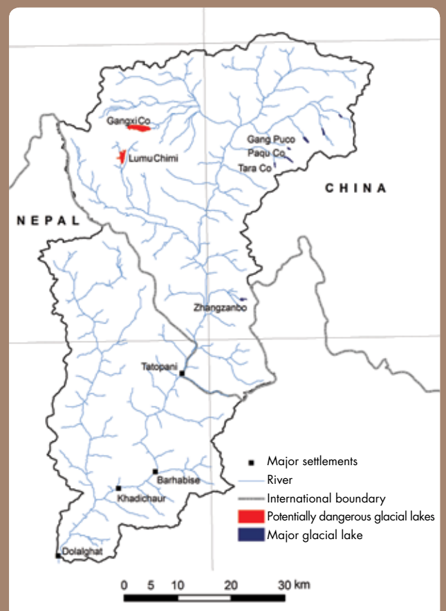
Figure 3: Major glacial lakes and potentially dangerous lakes in the Bhote Koshi/Sun Koshi basin
