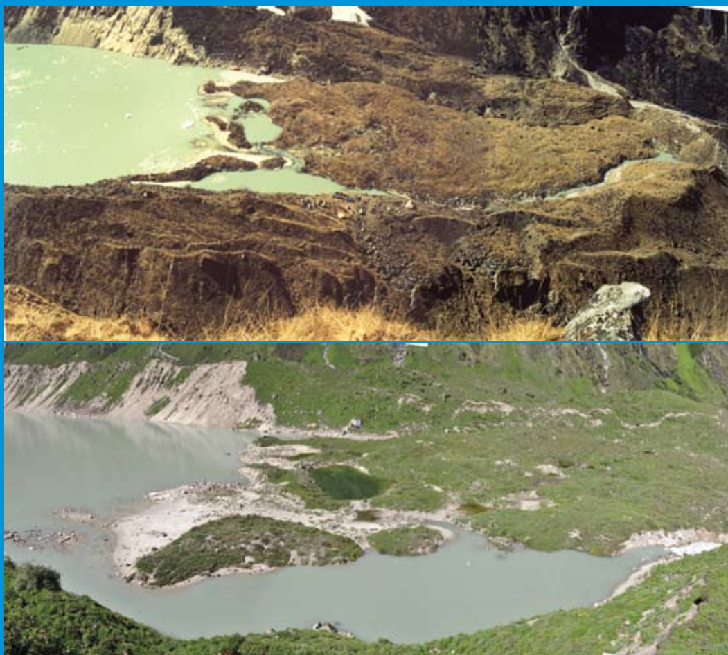
Figure 7.14: Changes in the shoreline of Thulagi Lake between 1996 (above) and 13 July 2009 (below), show the flow has now shifted towards the right lateral moraine, there are linear subsidence features on the left and right lateral moraines
