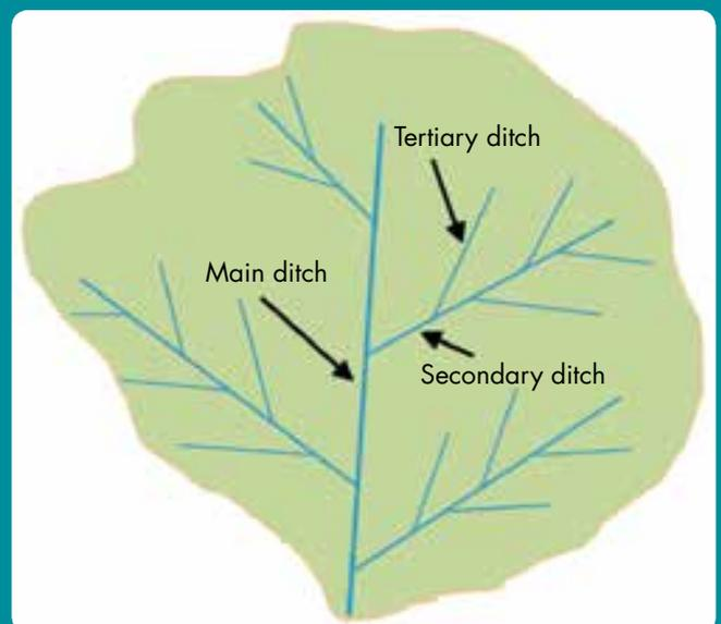
close as possible to its origin and channelled to a side drain, culvert, or any other nearby water course. Ditch excavation should start at the lowest point and work up in order that the accumulating water may drain off immediately. The most common types of drain are stone or gravel-filled drains with or without pipes.
