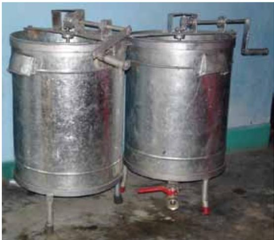
is then taken out, turned, and replaced to extract the honey from the other side. In a reversible extractor, both sides can be extracted without removing the frame. Stainless steel extractors give the best quality honey.
