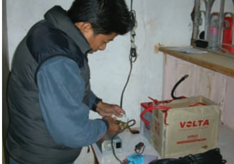
Installing a battery for a solar-powered computer system
