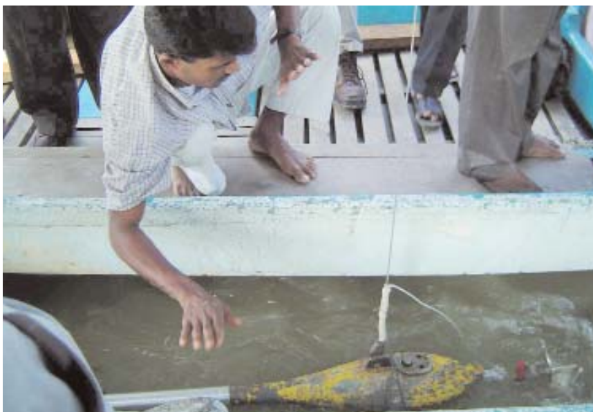
Discharge measurement in the Brahmaputra River at Bahadurabad, Bangladesh
