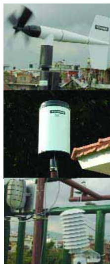
Nepal Climate Observatory (NCO) at ICIMOD and some of its instruments for measuring pollution levels
