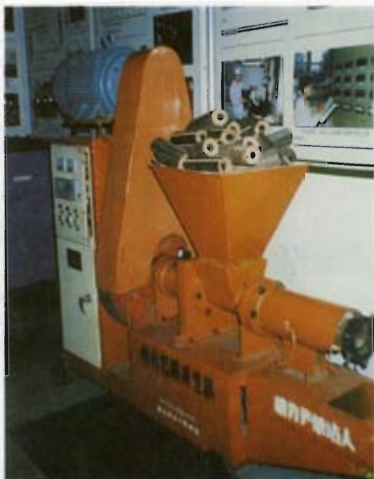
Small-scale biomass (agriculture residue) briquetting machine manufactured and being popularised in rural areas of China
