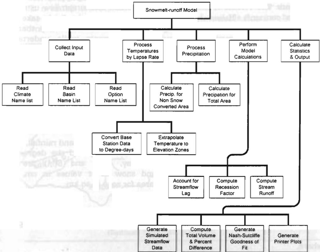
Fig. 1: Functional Flow Chart of the Snowmelt-runoff Model Computer Programme
