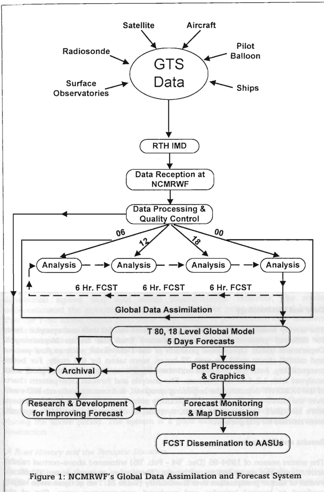
Figure 1: NCMRWF's Global Data Assimilation and Forecast System
