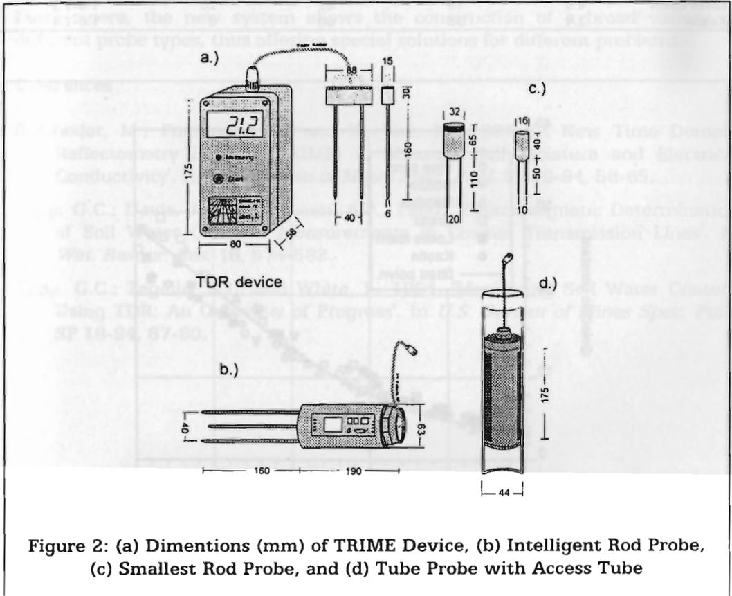
Figure 2: (a) Dimensions (mm) of TRIME Device, (b) Intelligent Rod Probe, (c) Smallest Rod Probe, and (d) Tube Probe with Access Tube
