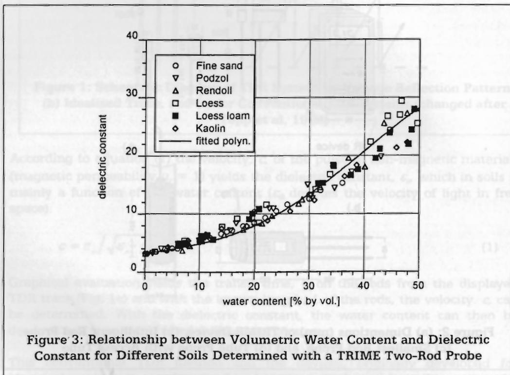
**Figure 3: Relationship between Volumetric Water Content and Dielectric Constant for Different Soils Determined with a TRIME Two-Rod Probe**
