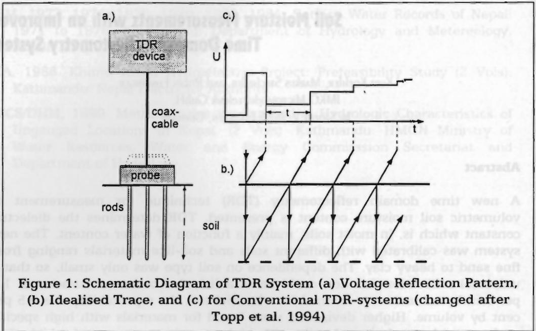
According to equation (1) the velocity,  $c$ , of the pulse in non-magnetic materials (magnetic permeability  $\mu_r = 1$ ) yields the dielectric constant,  $\epsilon_r$ , which in soils is mainly a function of the water content ( $c_0$  denotes the velocity of light in free space).
