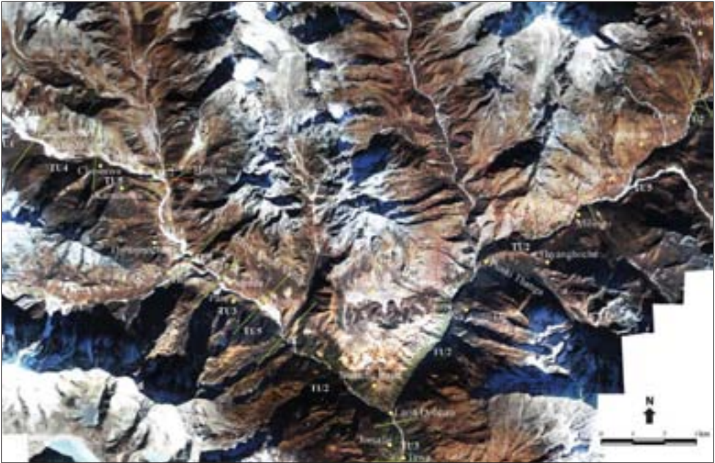
Figure 5.4: Terrain units (see Table 5.2) along the Langmoche valley and Bhote Koshi valley from Lake Dig Tsho to Namche Bazar (Larja Dobhan)
