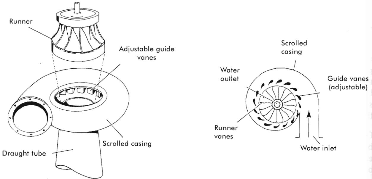
the speed of the generator is determined by the turbine, the speed of the turbine must be regulated (kept constant).
