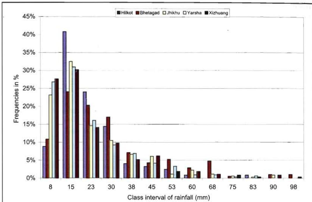
Figure 7.4: Rainfall frequency which generates runoff on erosion plots
