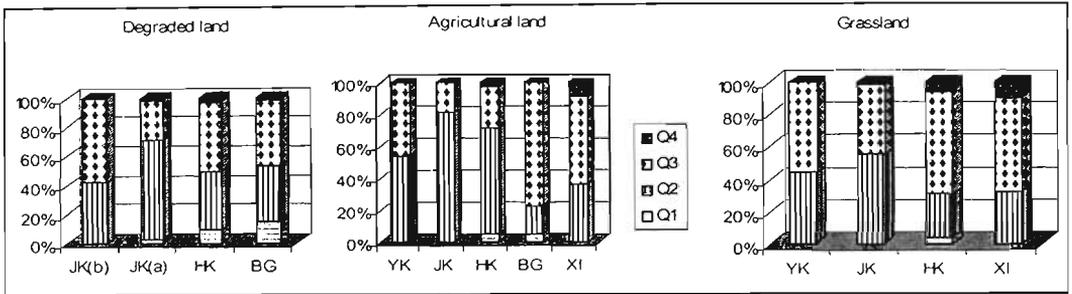
Figure 7.9: Quarterly distribution of soil loss from three types of erosion plots
