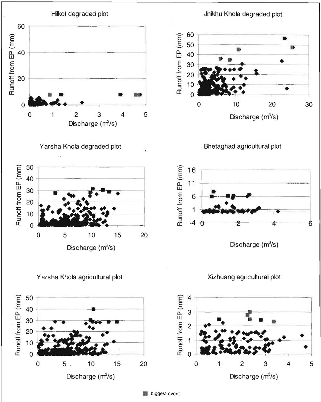
Figure 7.8: **Five biggest runoff events and runoff from erosion plot versus discharge at watershed outlets**
