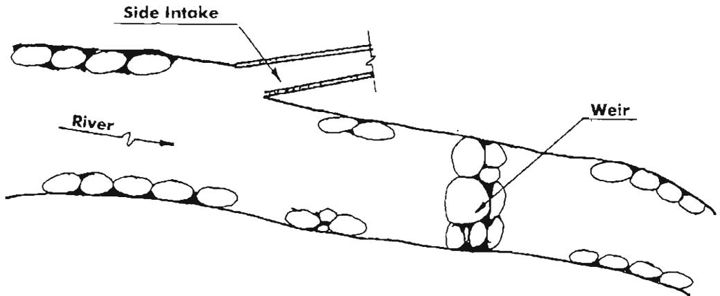
**Figure 5.1: Side Intake with Temporary Diversion Weir**
