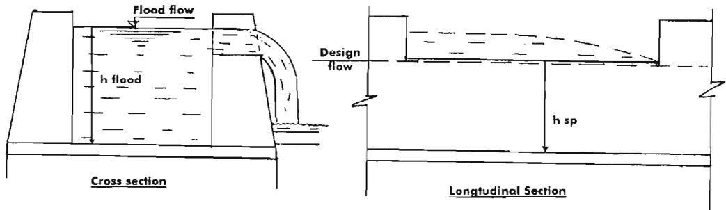
**Figure 5.4: Spillway Design**
