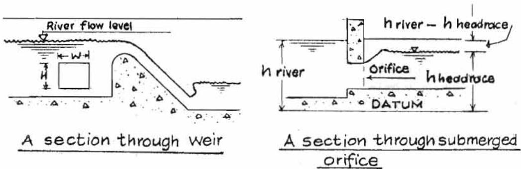
**Figure 5.2: Sections through a Weir and a Submerged Orifice**
