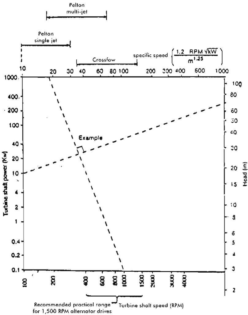
**Figure 5.11: Turbine Selection Nomogram**
