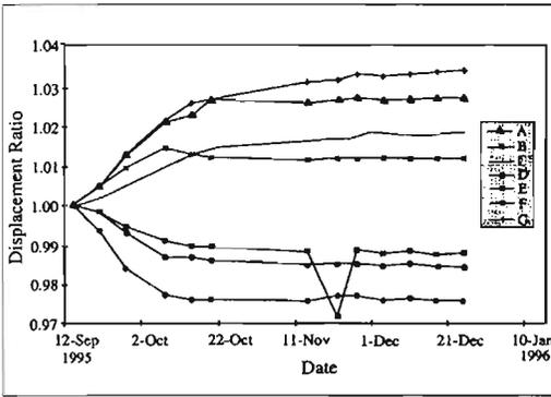
Figure 16.12: Displacement data obtained by the simple extensometers
