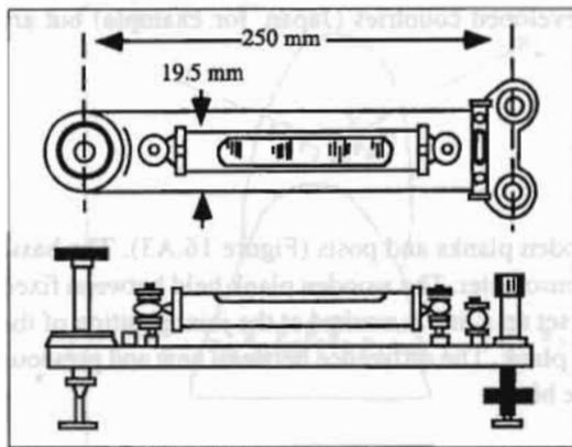
Figure 16.A4: A tiltmeter for measuring ground displacement
