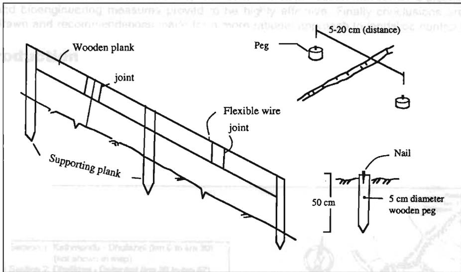
Figure 16.A3: Layout of a simple type A extensometer
