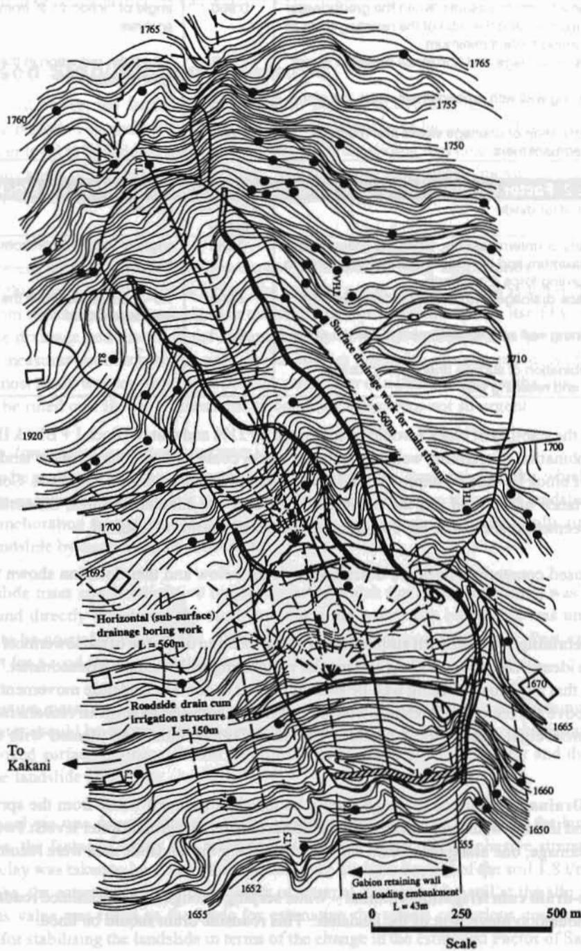
Figure 16.16: Map showing location of countermeasures proposed to stabilise the landslide
