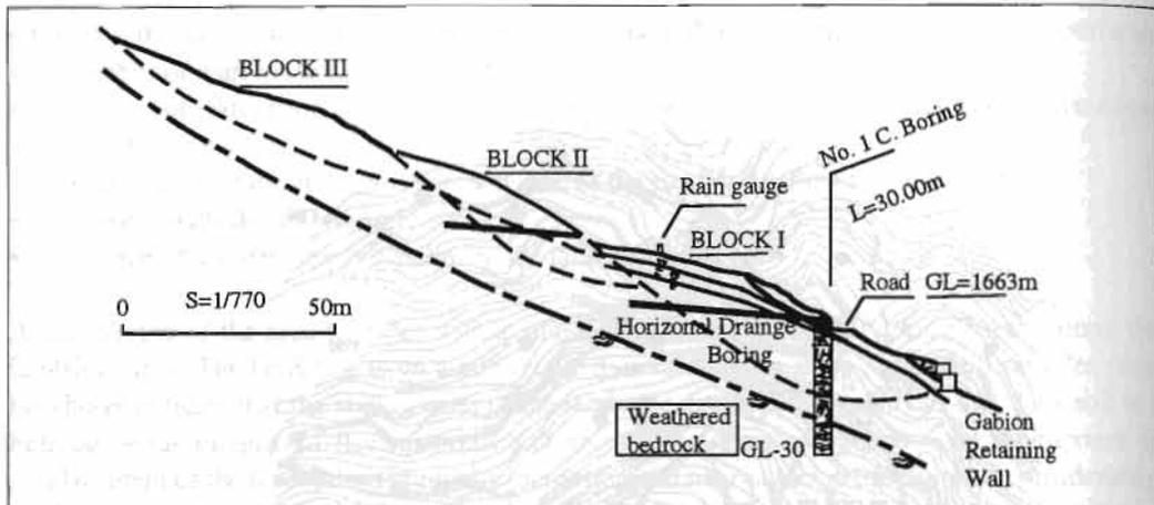
Figure 16.3: Cross-section of the landslide showing the subdivision into different blocks
