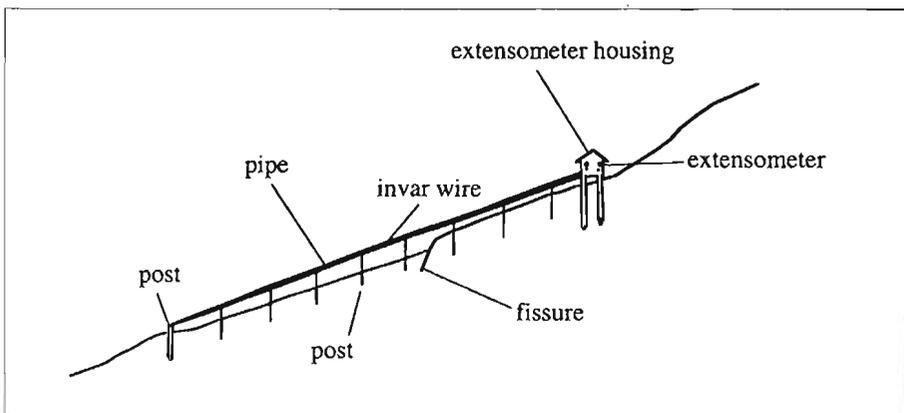
Figure 16.A2: An automatic extensometer
