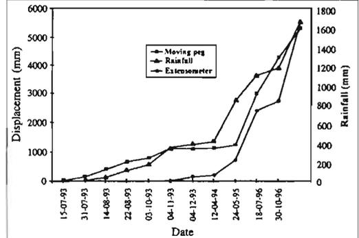
Figure 16.15: Relationship between the displacement shown by pegs and extensometers and rainfall (cumulative)
