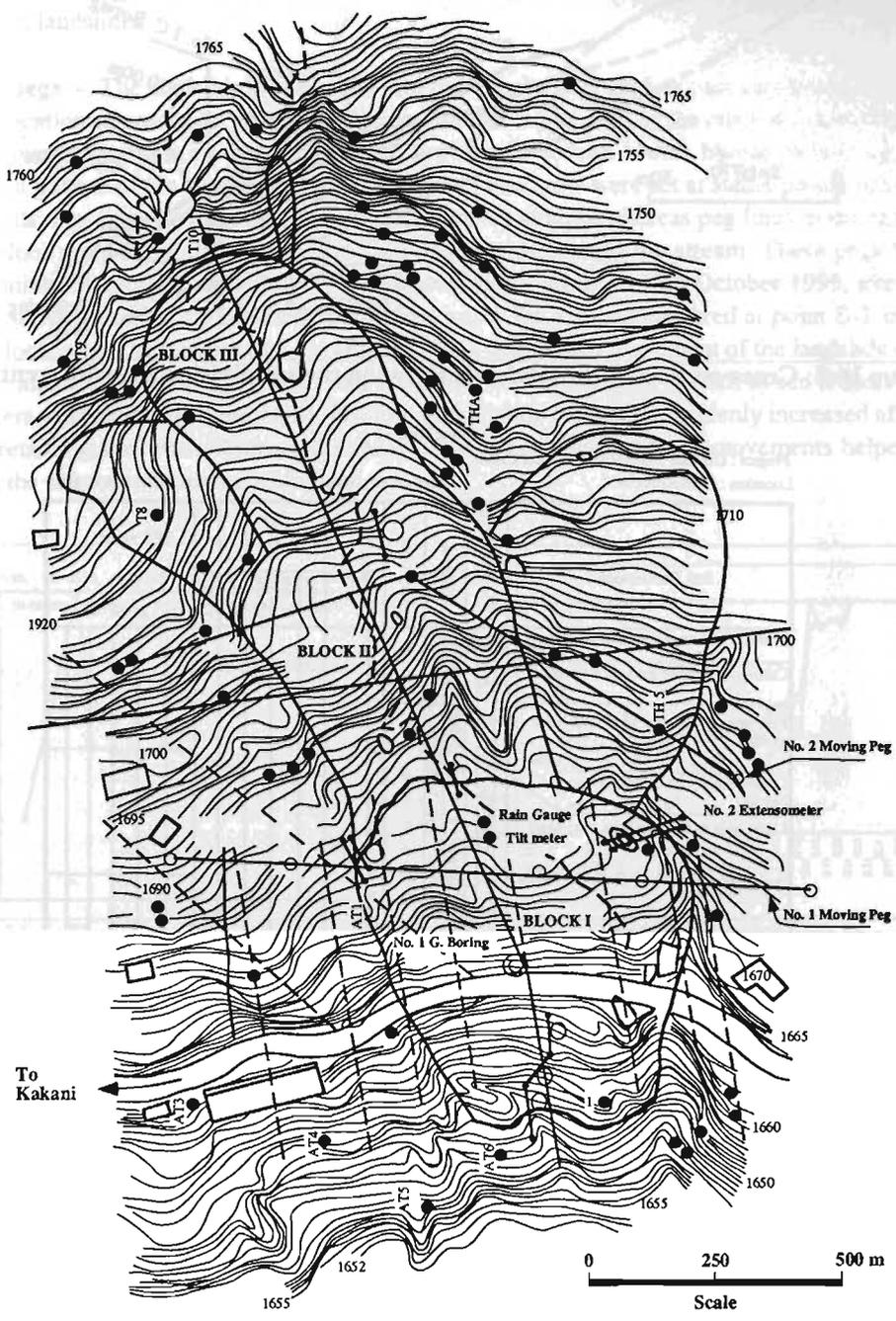
Figure 16.2: Topographic map of the landslide area and location of monitoring equipment
