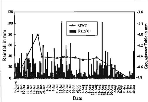
Figure 16.14: Relationship between rainfall and the groundwater table
