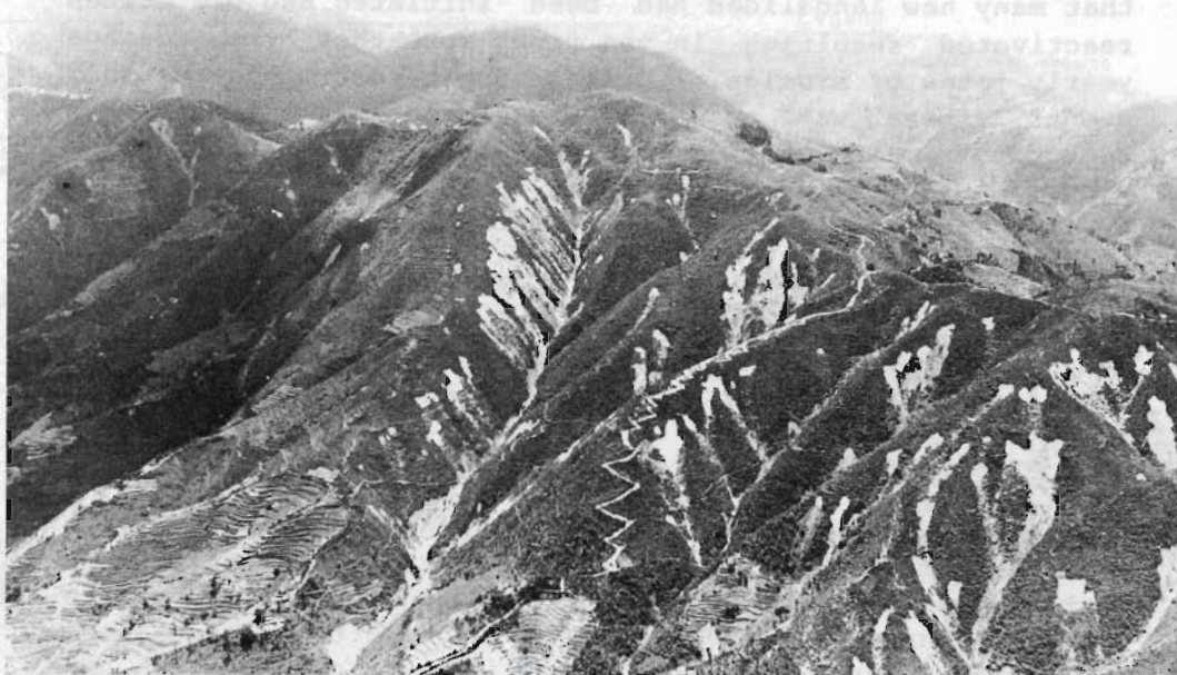
Photo III Near Lele, Lalitpur District. After a prolonged rainfall in Sept. 1981, this slope failed en masse in spite of thick shrub cover. Such catastrophic events are common on certain landforms within the Nepal Himalayas but are difficult to predict.
