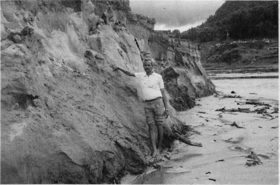
Figure 9. Kulekhani Reservoir Delta. Headcutting of sand and gravel deposit during low stages of the reservoir. The deposits are primarily sand with gravel lenses near the top (June, 1994).
