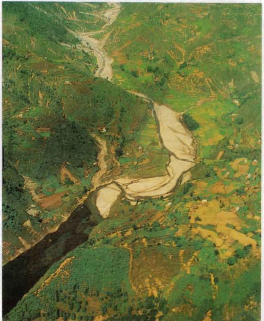
Figure 1. Kulekhani Reservoir - Coarse bed-material (cobbles, gravel and sand) are shown as a deltaic deposit at the upstream end of the reservoir. The delta is about 2 km long and floating debris is seen adjacent to the delta. The Bisingkhal Khola delta is shown at the bottom right side of photo (September 1993).
