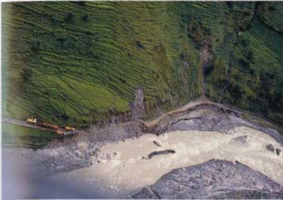
About one fourth of this road was severely damaged by a glacial lake outburst flood (GLOF) in 1981, Arniko Highway, Nepal.
