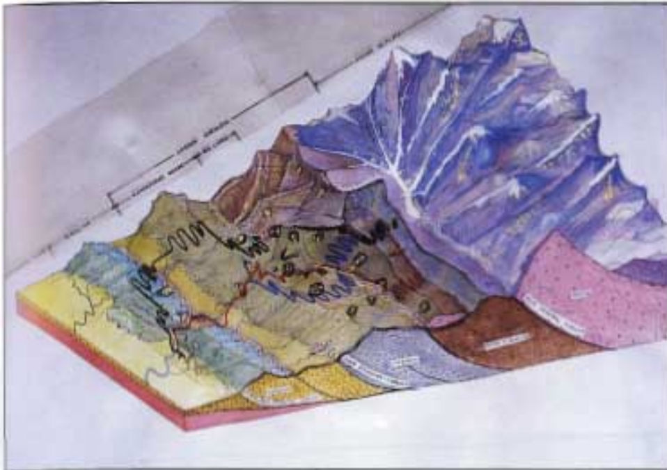
Idealized cross-section of the Himalaya showing valley road and ridge road
