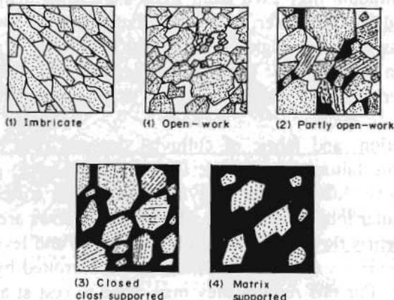
Fig. 1.4 Fabric of colluvial materials
