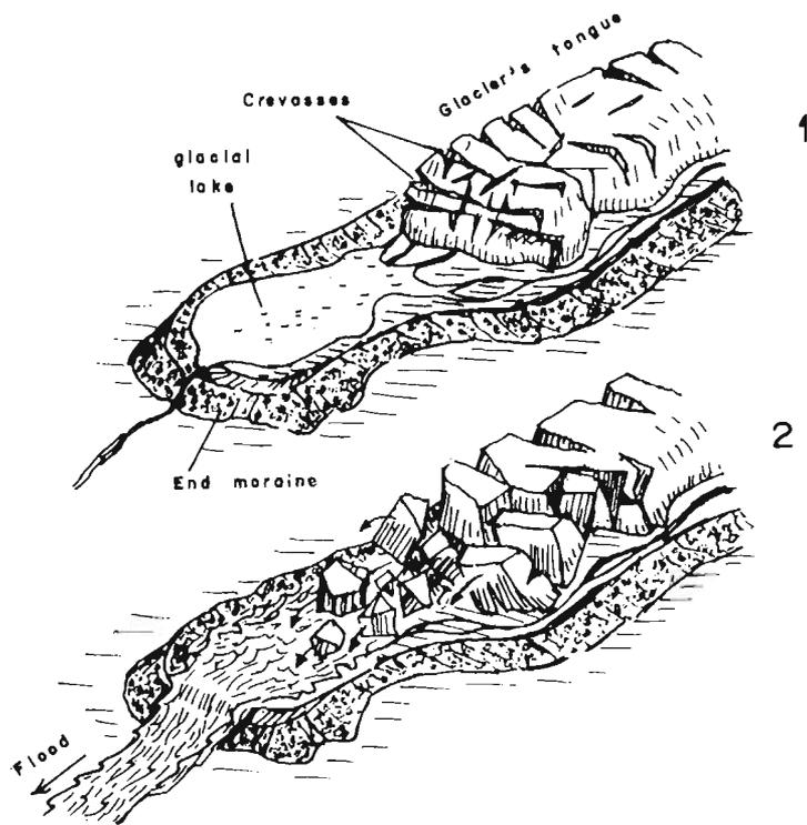
Fig. 1.14 Common mechanism of a glacial lake outburst flood (GLOF) in the *Himalaya*
