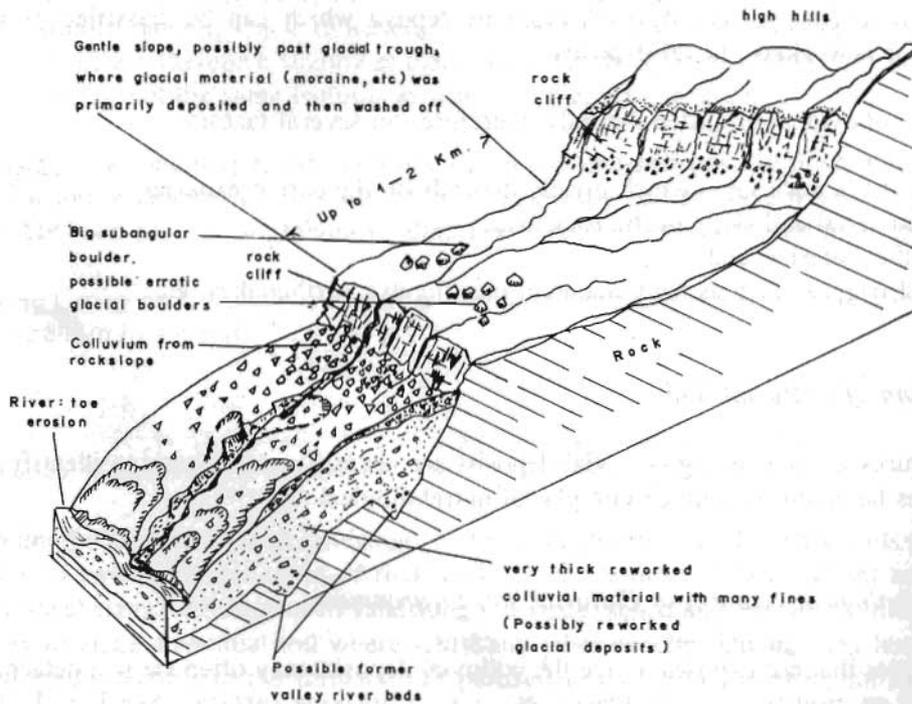
Fig. 1.3 Features of reworked colluvial or reworked glacial deposits and their environmental morphology
