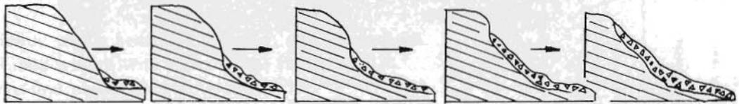
Fig 1.5 Richter Slope: A hypothetical rock slope angle lowering process with formation of a colluvial deposit
