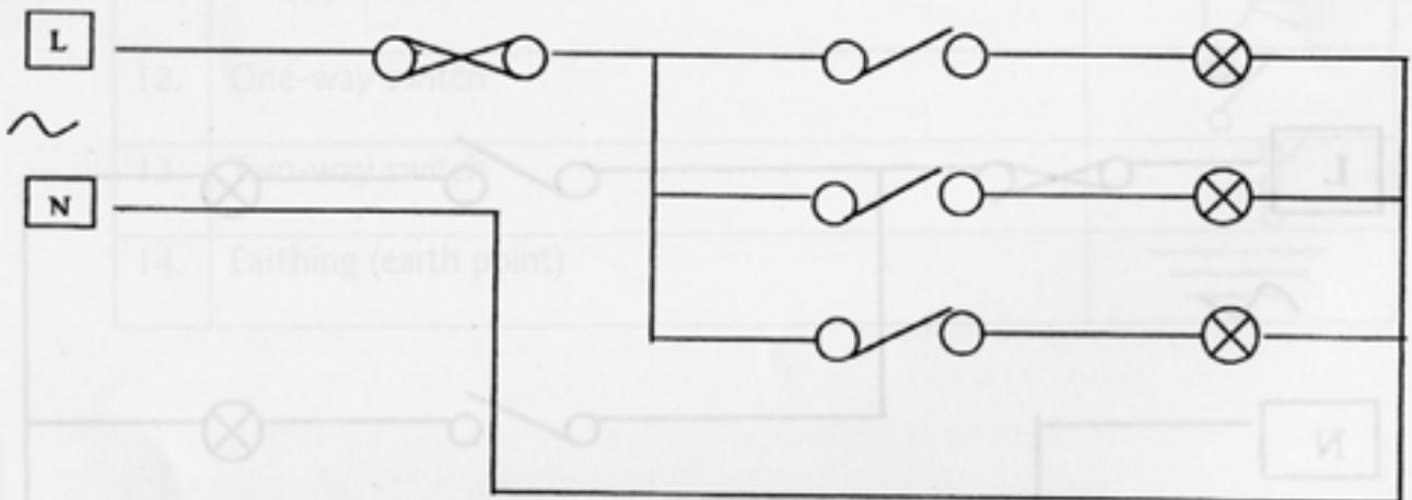
**Figure 4.7: Circuit with Three Lamps Controlled by Three Separate One-way Switches and a Double Pole (DP) Switch, with Fuse. The DP Switch is Useful if a Sub-circuit Needs to be Disconnected from a Different Location**
