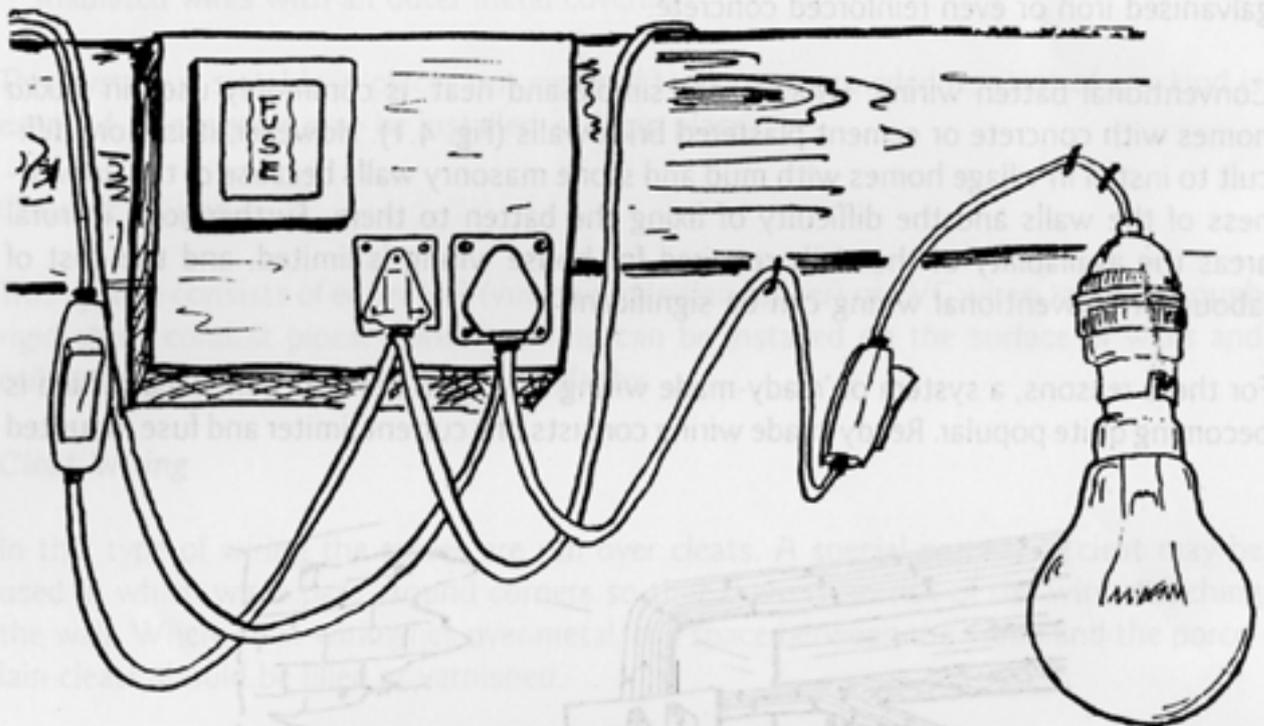
**Figure 4.2: A Ready-made Wiring System**
