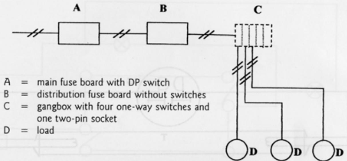
**Figure 4.13: Block Circuit Diagram for House Wiring**
