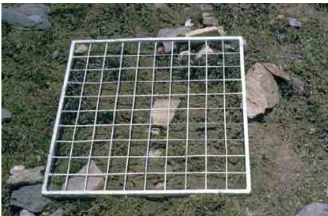
Figure 3.2: Quadrat method for estimating surface material and vegetation cover
