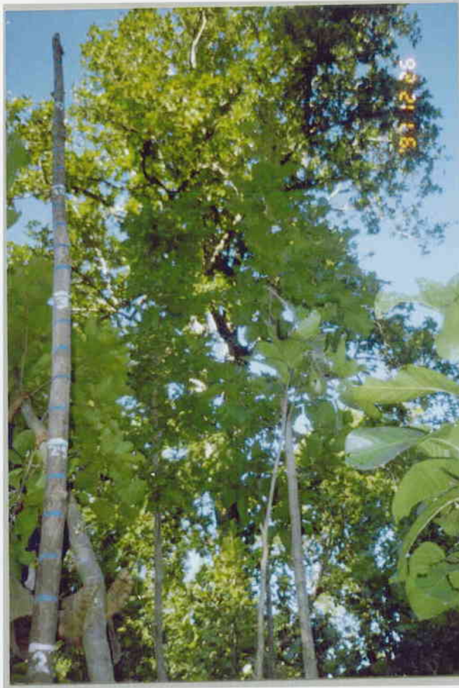
Figure 3.12: Height measuring pole
