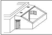
Backside of the roof is supported either by the backside wall, or by a thin beam for an attached shed. First is a layer of twigs, that is then covered by dry grass or cardboard, recovered then by mud.
