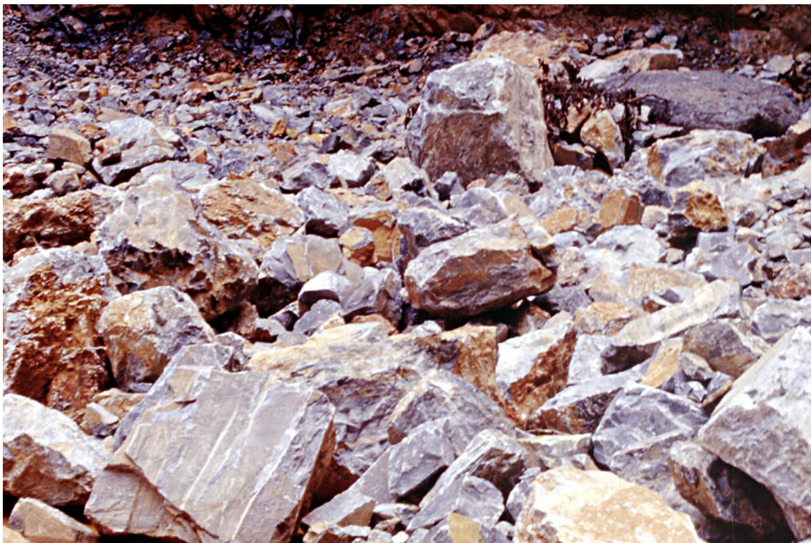
Plate 16: Extracted limestone from the quarry site used as raw material for cement factory.
