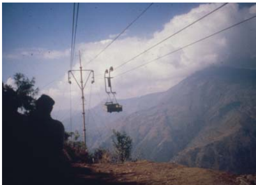
Figure 6: Hydro-powered ropeway transport system ©Practical Action
