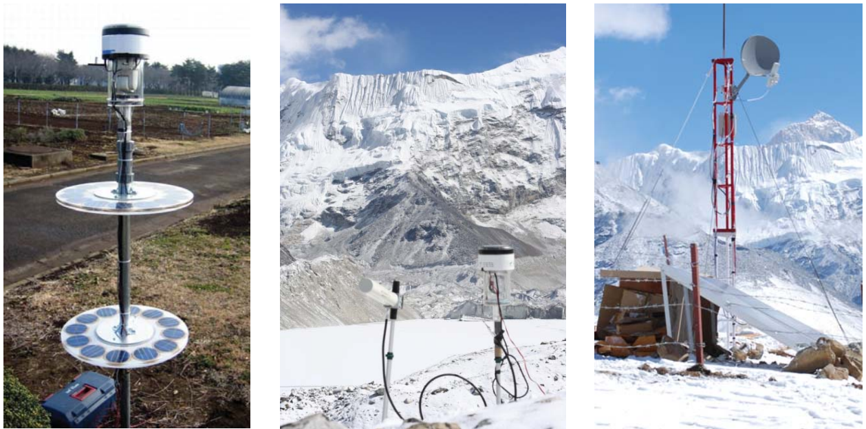
Figure 6: Field server equipped with web-camera enclosed within a protective shield (left) installed close to the end moraine of Imja Tsho (middle). On the right is the transmitting station.
