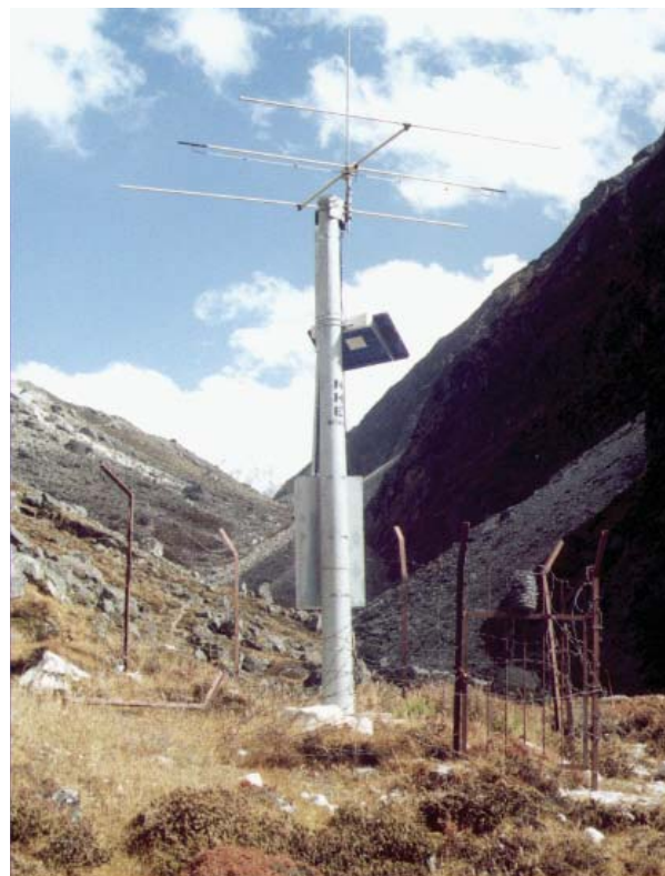
Figure 4: Components of Tsho Rolpa TEWS: the transmitting station at Sangma Kharka outside Tsho Rolpa (left) and warning installation (right).
