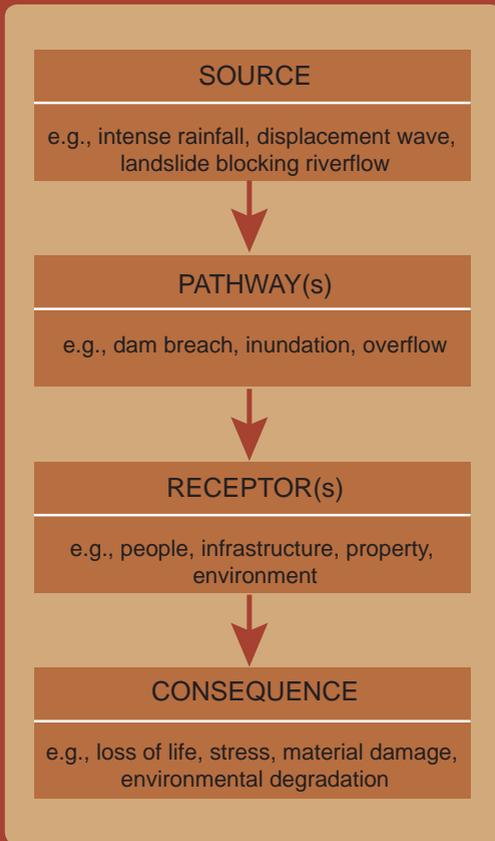
Figure 3: Procedural diagram for flash flood risk analysis
