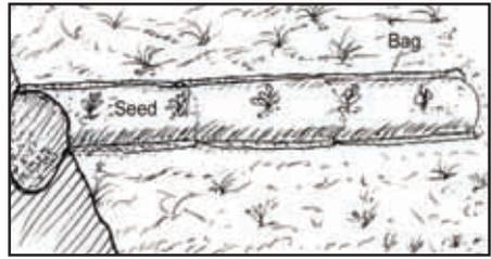
**Earthen and stone V-shaped bunds.** A direct derivation of the traditional bunds found in the lowlands, these structures are intended to check the movement of soil and gravel through the downward movement of melting snow and to increase the time available for water to percolate through the soil. Such bunds are usable for steep areas and are shaped into a ‘V’ to cushion the snow’s weight as it rests across a smaller surface area. ‘V’ bunds also reduce the danger of uneven water
