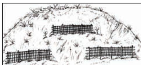
stems/trunks have not started to grow in the soil. Seeds can be placed behind the structures to add both to the stability of the structure and increase biomass cover in the area. A metal mesh can also be added to the structure to give it additional strength.
