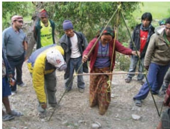
Step 2: How to locate contour lines using an A-Frame
