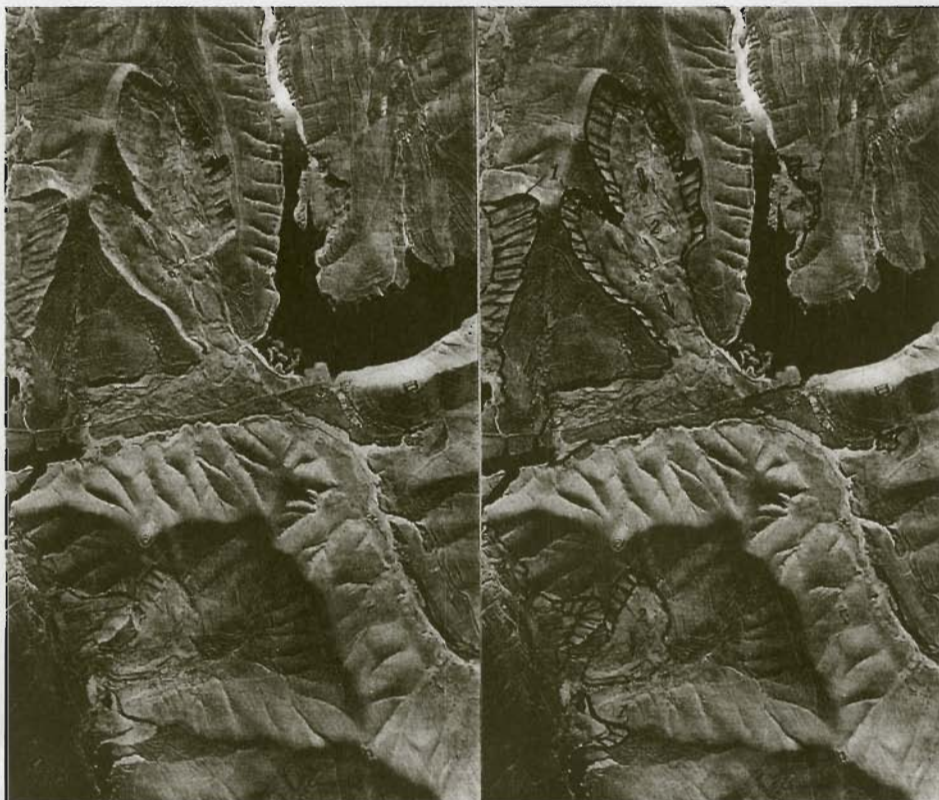
Plate 2: Aerial Photography (left) and Interpretation of the Aerial Photography (right) to Identify the Geomorphic Features of Landslides in Haiyuan Area, Ningxia 1 - Main Scarp; 2 - Slide Mass
