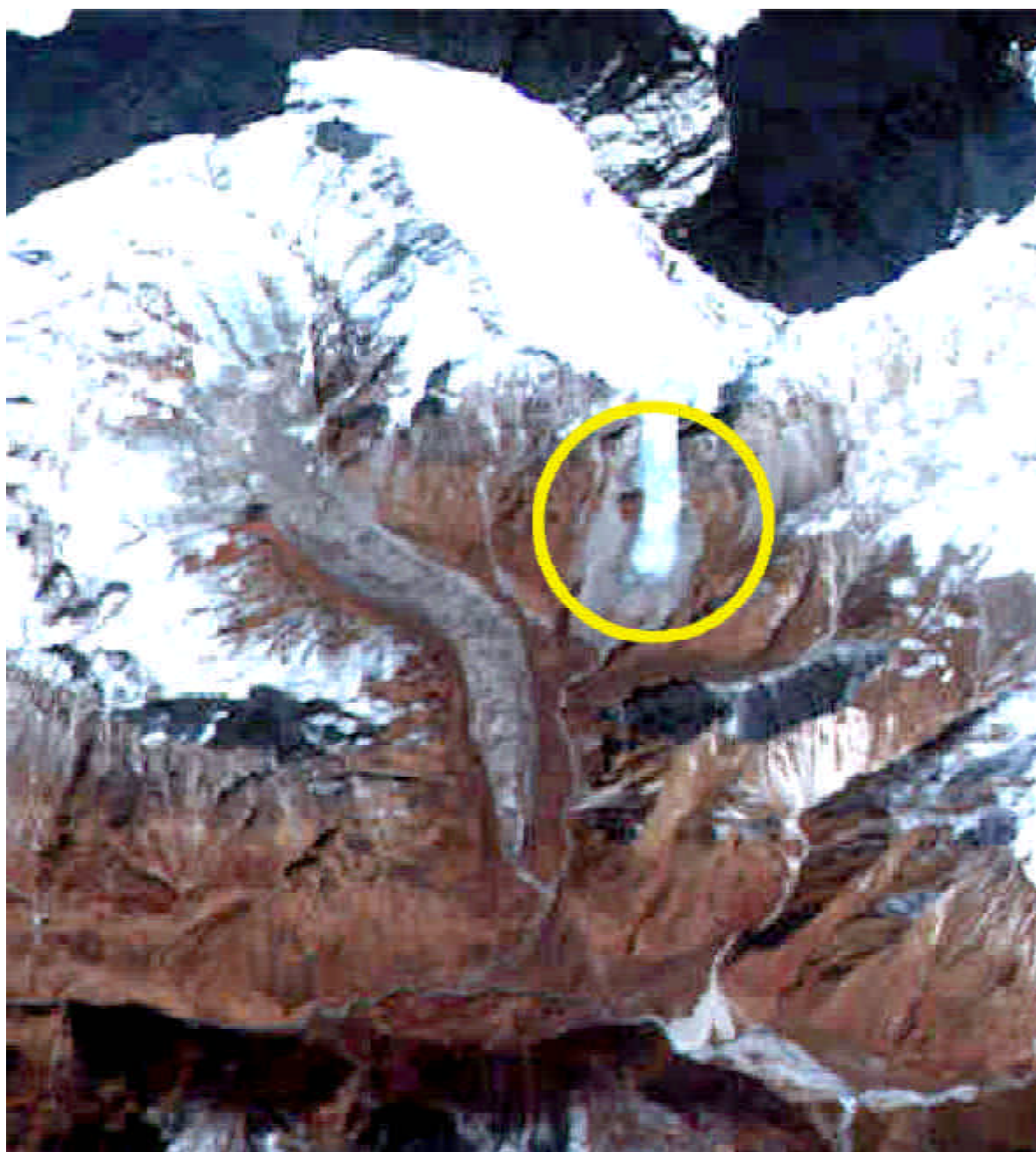
Figure 6.14: IRS1D LISS3 FCC R3G3B2, 3 January 2000, showing evidence of the past GLOF from the end moraine dammed glacial lake associated with the hanging glacier of Lirung–Kyenging Glacier in Langtang Basin in Nepal
