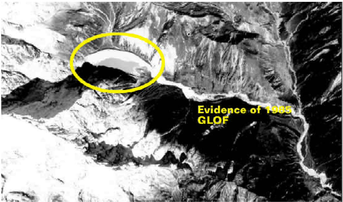
Figure 6.23: Part of an aerial photograph of 1992 acquired by the Survey Department of HMGN showing Dig Tsho Glacial Lake and the effect of the 1985 GLOF (Aerial Photo 52-49)
