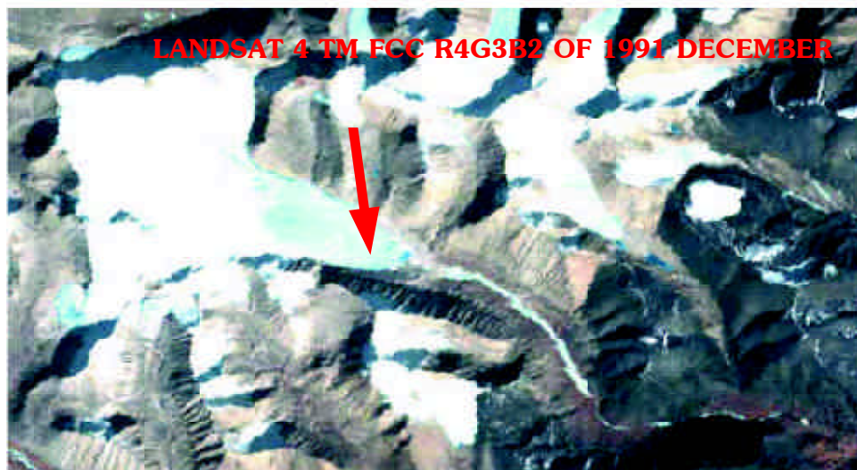
Figure 6.18: Satellite images of 1999 and 1991 showing evidence of a past GLOF event before 1991 from the lake at the tongue of Glacier Gr_207 in Kali Gandaki basin. The breached lake is not refilled.
