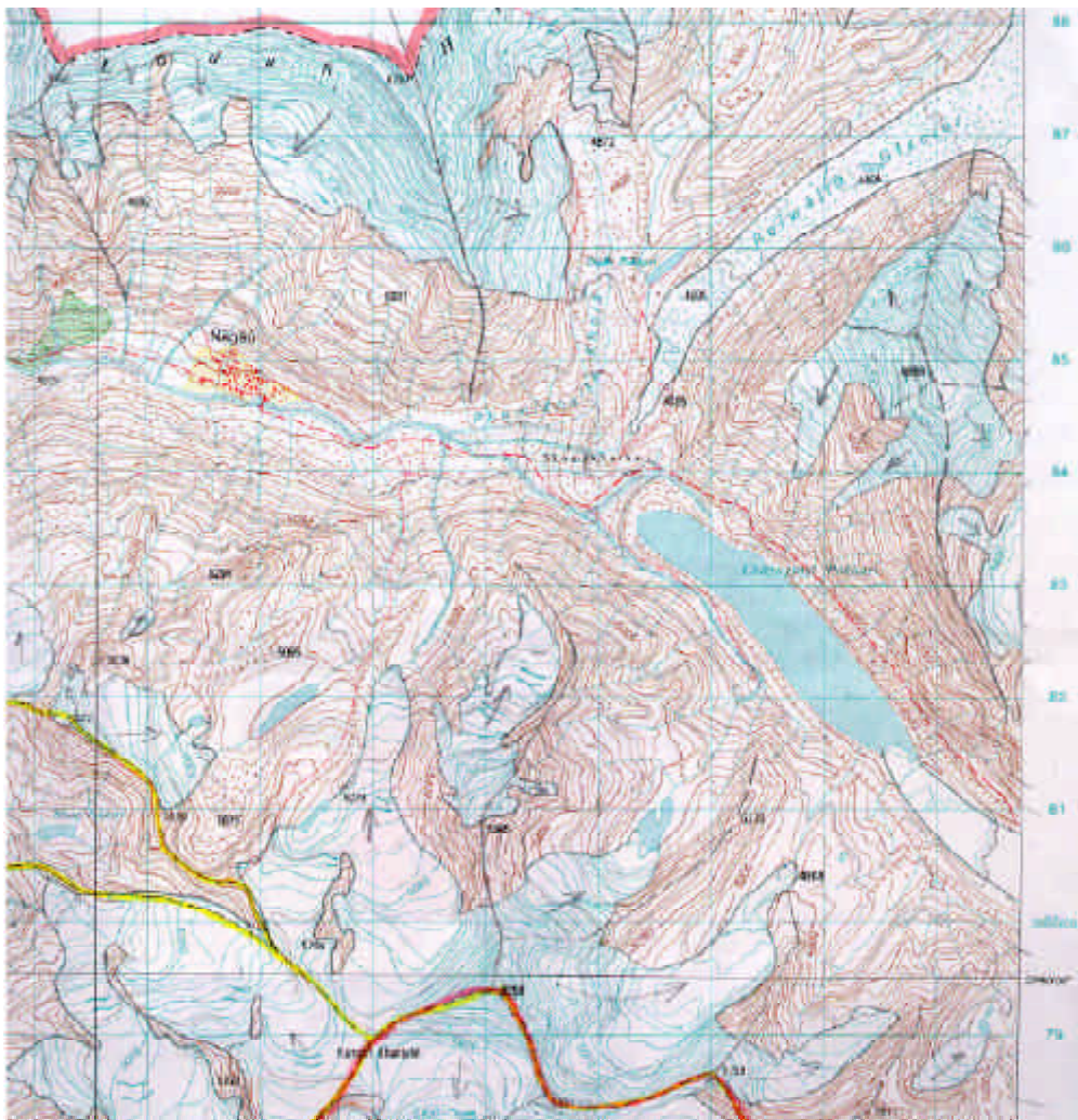
Figure 10.29: Part of the topographic map of Rolwaling area published in 1996 by the Survey Department of HMGN on a scale of 1:50,000 based on aerial photos of 1992 and field verification in 1996
