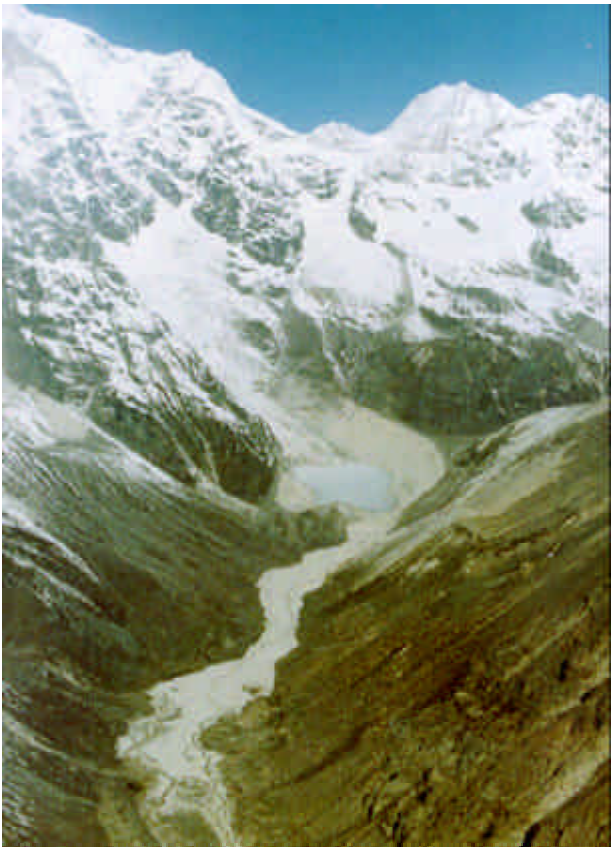
Figure 9.17: Birds-eye view showing the remnants of Dig Tsho Glacial Lake, Langmoche Glacier at the slope and the debris along the gully after the GLOF of 1985 (WECS 1991)
