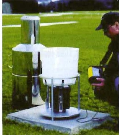
d) PLUVIO 1000 mm with collecting-ring heating device
