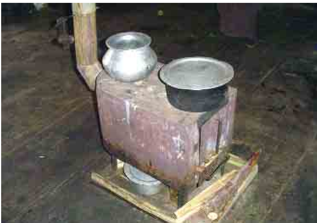
Figure 4.1: Modified bhukhari type stove in Bhutan
