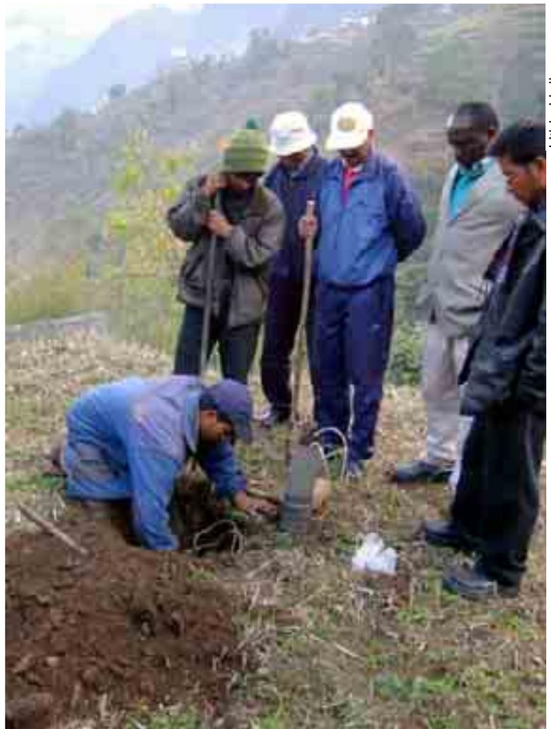
**Measuring nutrient losses caused by leaching at Landruk**
