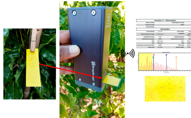
Figure 5. Wireless DropletScope ® System.
