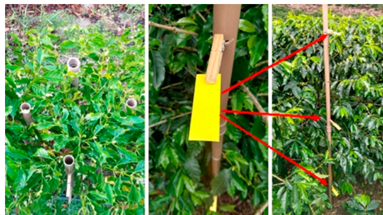
Figure 4. Arrangement of water-sensitive paper tags using PVC templates.
