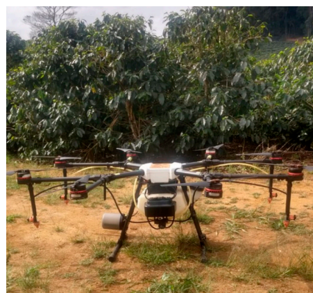
Figure 1. Multirotor unmanned aerial vehicle used for spraying in the experiment.
