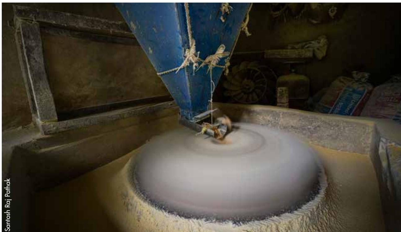
Rural communities in Nepal still operate traditional water mills for basic mechanical work. Three traditional water mills were operated by their owners in Mathillo Dhand, Karamfedi, and Ratamate. Operating on the kinetic energy of rivulets, these water mills are used by the owners for processing grains. Villagers also offer remuneration or a portion of the ground grains for use of the water mill. However, these mills and their water canals were damaged beyond use during the earthquake.
