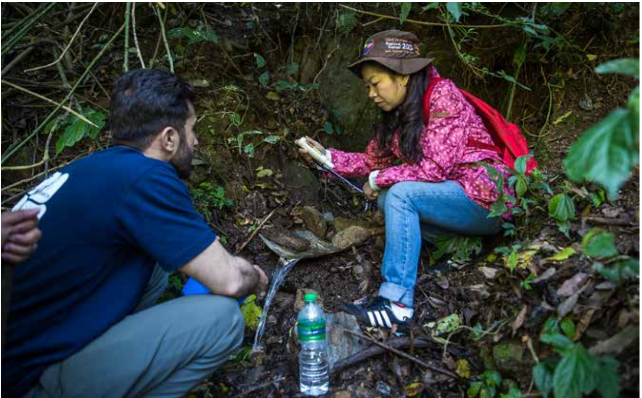
Participants conducting discharge and water quality measurements at Sungure Khola spring.
